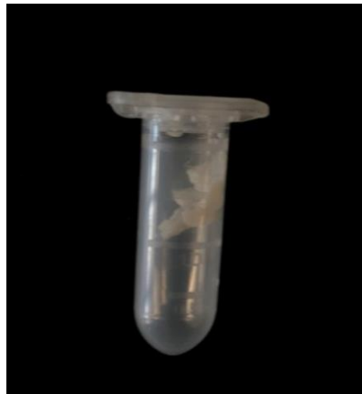
Figure 4: Scale Scraped Down from Vessel
