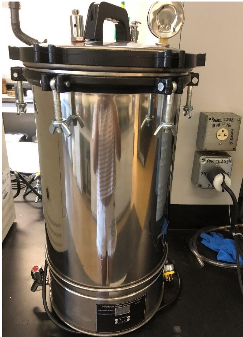
Figure 8: Pressure Vessel Used to Stimulate Boiler Conditions
